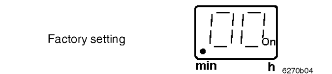
Fig. 12-5 Factory setting of pause time "P2" (minutes)
